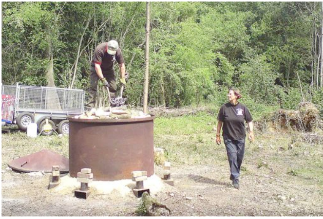
Rob ignites the timber by pouring burning embers down into the centre of the kiln.
