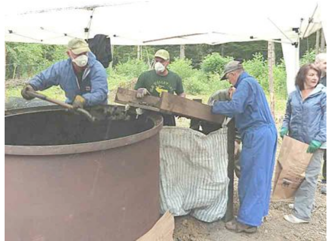
The dirty job of shovelling the charcoal over a sieve and into sacks.
